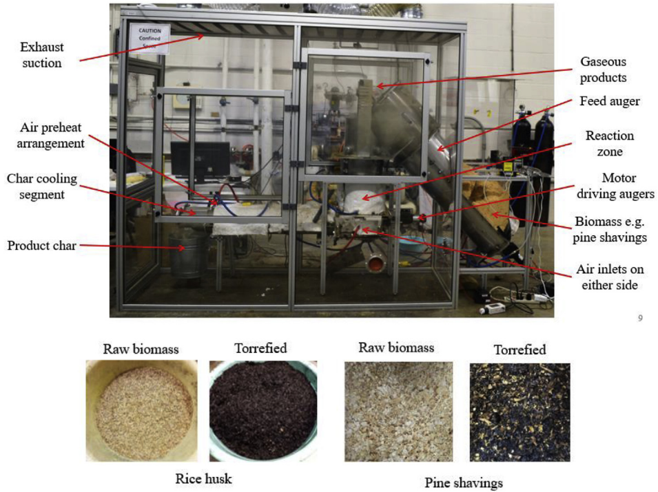
Fig. A1. Experimental set-up of pilot-scale moving bed reactor in laboratory, and the pictures of the biomass samples.
