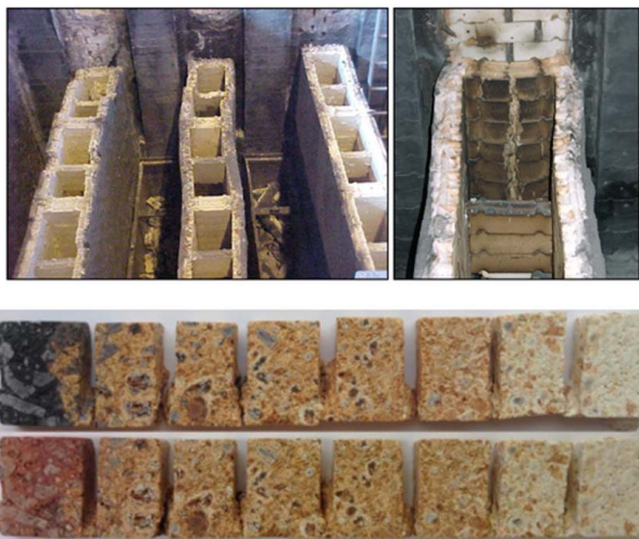
Fig. 2 Deterioration of refractory materials properties due to aging effects [29]
