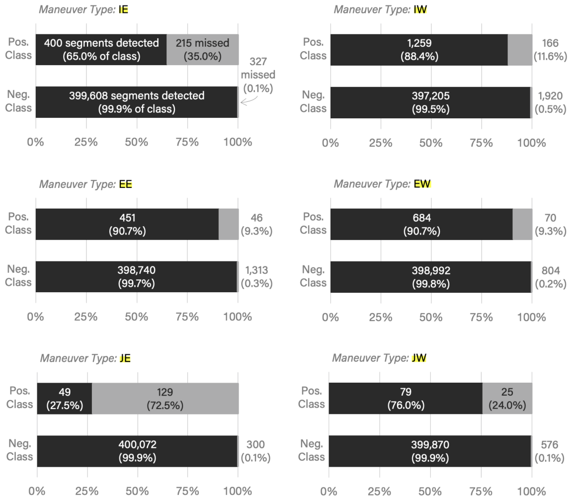
Figure 4-2: Performance metrics for the suite of satellite maneuver detection algorithms on a segment-by-segment basis after training on five years' worth of GEO satellite data. The true positive and false negative portions of the confusion matrices are shown in the positive class of each bar chart in black and gray, respectively. The true negative and false positive portions of the confusion matrices are shown in the negative class of each bar chart in black and gray, respectively.
