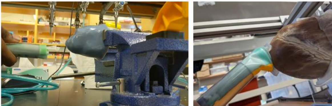
Figure 18: Left. Delivery tool deployment using 3D printed systole heart model, with initial frame concept. Right: Deployment using fixed porcine heart with developed vacuum frame components
