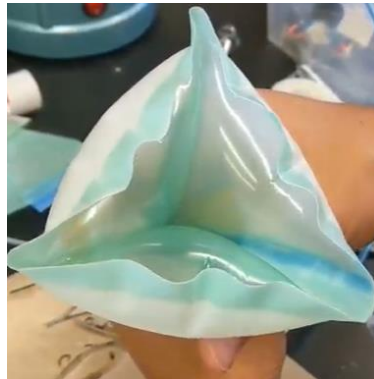
Figure 8: cut-out, folded and bonded delivery sleeve, central enclosed space completely occluded by inflated region
