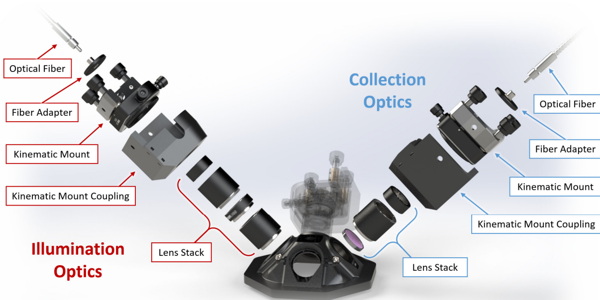
Figure 3-6: An exploded view of an example configuration of the optical probe head. Signal is transmitted to the kinematic mounts via optical fibers. That signal is then aligned via the kinematic mount and coupling assembly so that the light can be filtered and tuned as it is directed to and from a sample.
