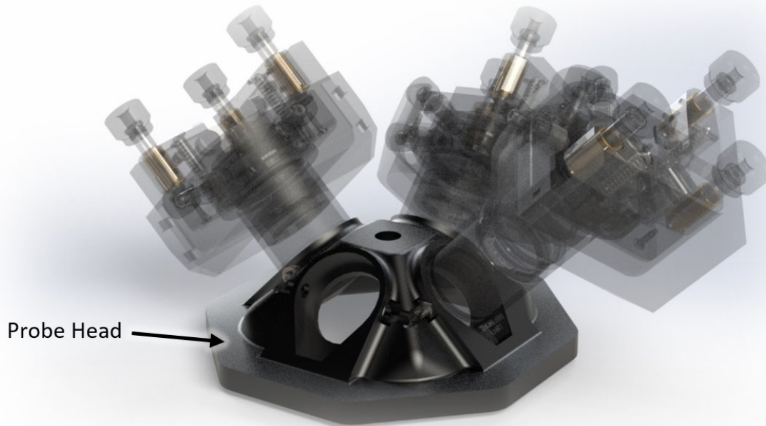
Figure 4-1: Rendering of the optical probe head assembly with the probe head labeled. The optics are displayed semi-transparent to more easily identify the probe head.
