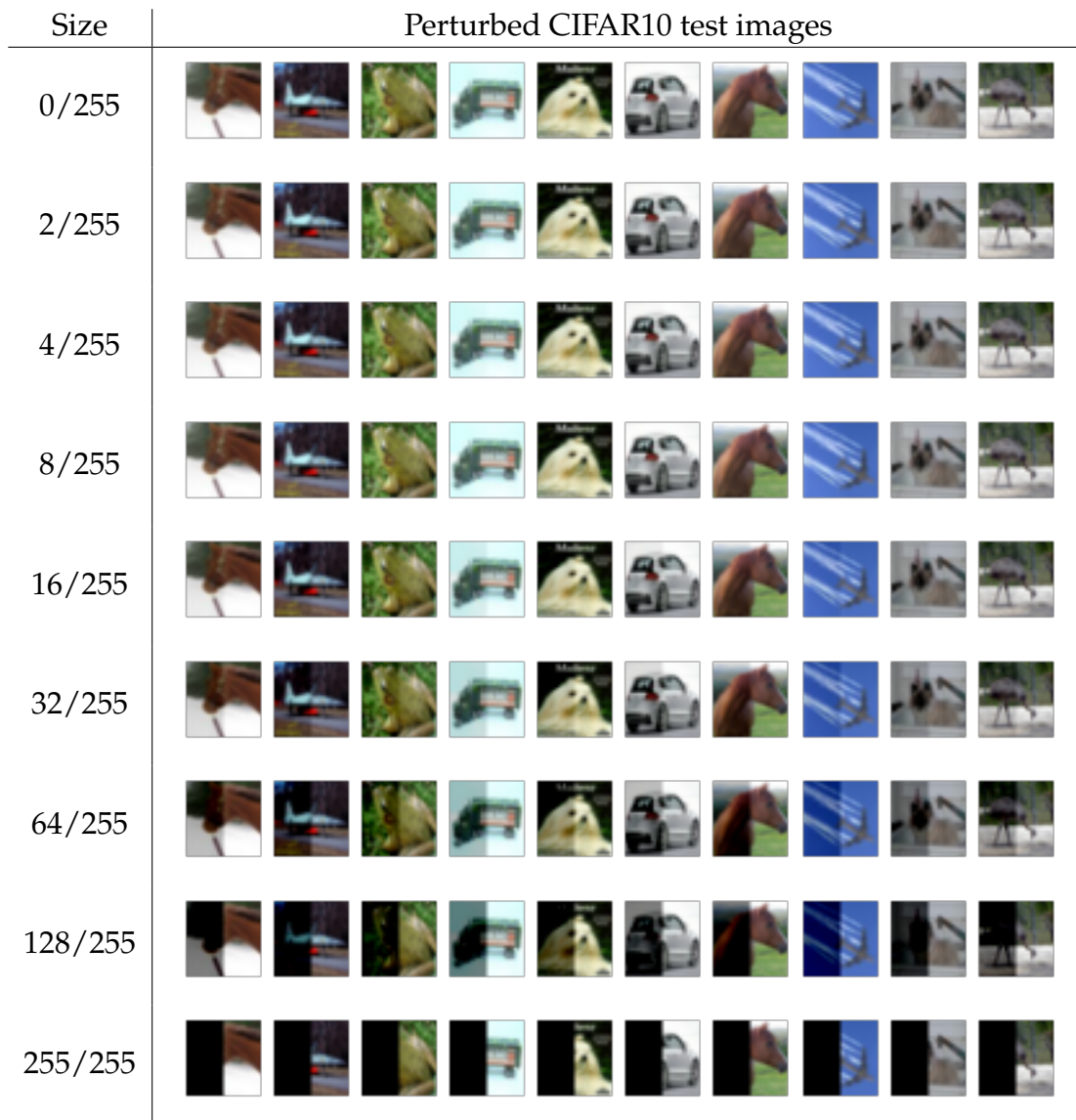
Figure 1.0.2: Visualization of different levels of pixel perturbations on CIFAR10 images. The images are the first ten images of the CIFAR10 test set. For each perturbation size \epsilon , the pixel intensities in the left-half of each image are decreased by \epsilon and clipped to zero if they go negative. A maximum perturbation of size 255/255 results in an completely black left-half. Note that a perturbation of \epsilon = 8/255 is near-imperceptible.
