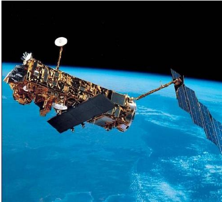
Figure 3-1: An illustration of Envisat, a large, defunct satellite that is exhibiting a uncontrolled tumble while residing in a high-density LEO orbit. Image credit: European Space Agency.
