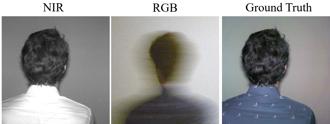
Figure 3-10: Some materials have visible patterns but uniform NIR reflectance. For these materials, the reconstruction problem is equivalent to plain de-noising or de-blurring. Since our network is trained to extract high frequency information from the NIR image, it is not able to reconstruct textures that are neither visible in the NIR nor the RGB image.
