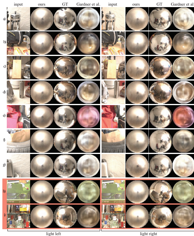
Figure 2-5: As the first application of our dataset, we train a deep network to predict environment maps from single input images. Our model consistently predicts the dominant light direction of the ground truth environment map. The model successfully estimates illumination based on shiny objects (a and g) and diffuse reflectors (e.g. row f). Rows h) and i) show failure cases where the network predicts low-confidence outputs close to the mean direction. We compare to Gardner et al. ’s algorithm [14] which, while predicting visually plausible environment maps, lacks the precise localization of highlights shown by our technique. (Please ignore the vertical seam in Gardner et al. ’s result. Their model uses a differing spherical parametrization, which we remap to our coordinate system for display.)
