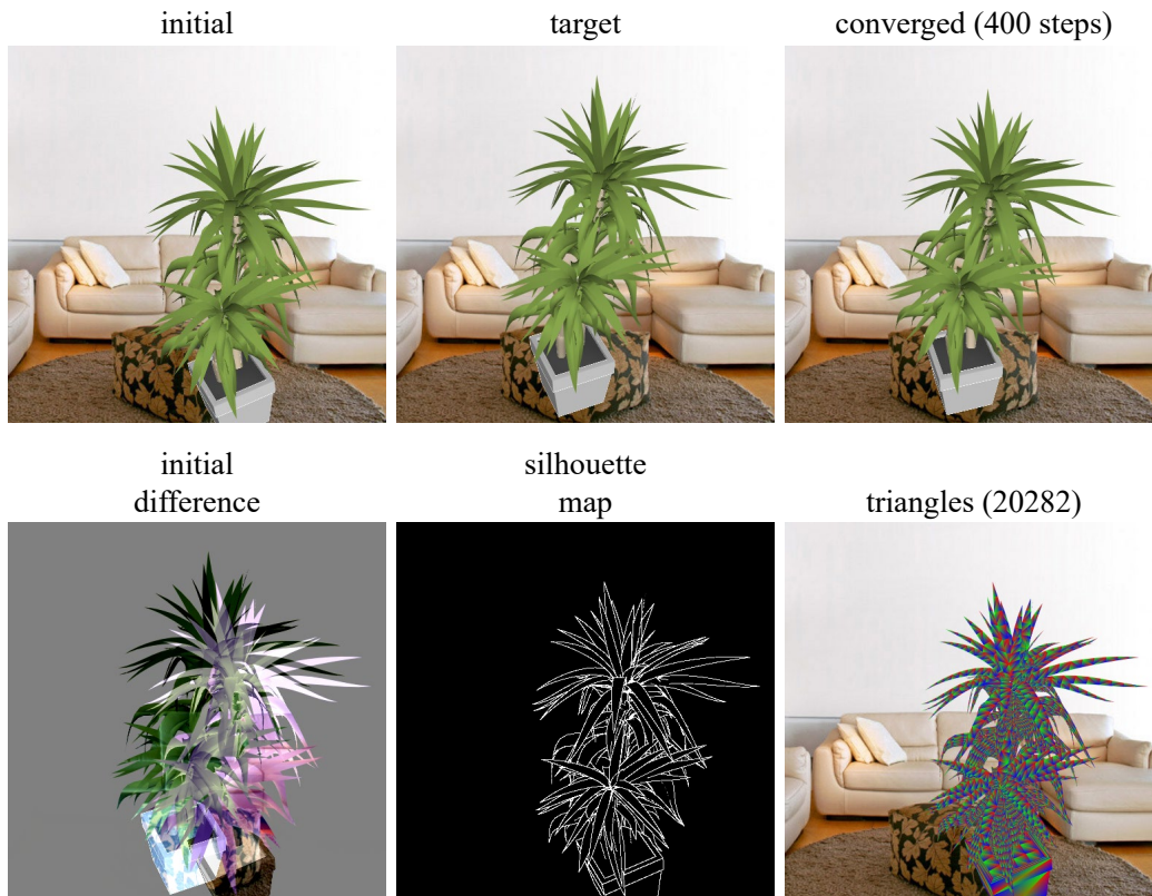
Figure 4-16: 6 DoF pose estimation for a scene with high triangle count and significant depth complexity. A combined forward/backward pass for this model with more than 20,000 triangles takes less than 13ms.
