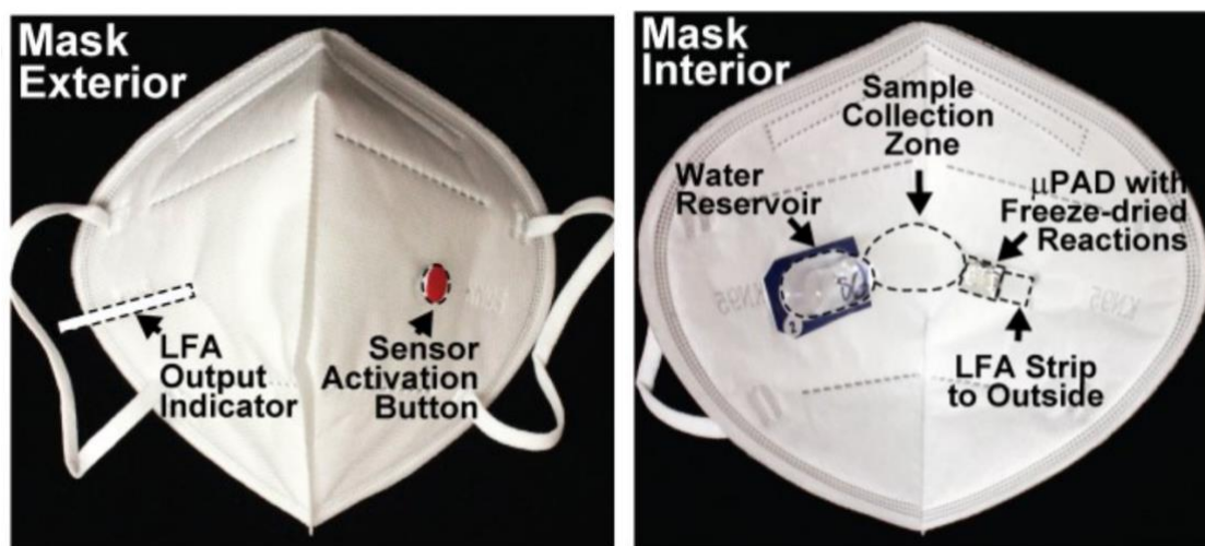
Figure 3-16. Photographs of the SARS-CoV-2 sensor integrated into a face mask. Shown from the exterior angle (left) and the interior angle (right). Details of device function can be seen in Figure 3-15.
