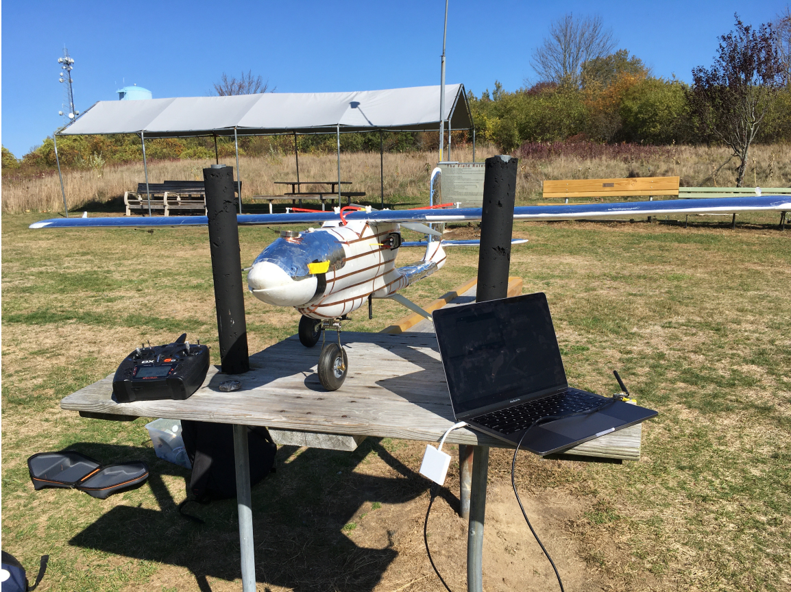
Figure 2-2: Plane with aluminized Mylar and copper tape configuration.
