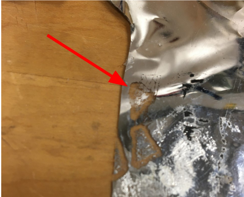
Figure 2-3: Aluminumized Mylar melted at the connection to the copper tape.
