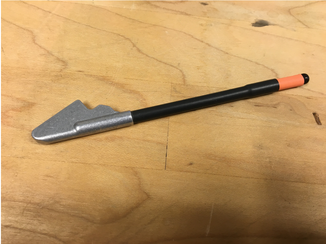
Figure 3-1: Standard p-static discharger wick used on commercial aircraft, manufactured by Dayton-Grainger.
