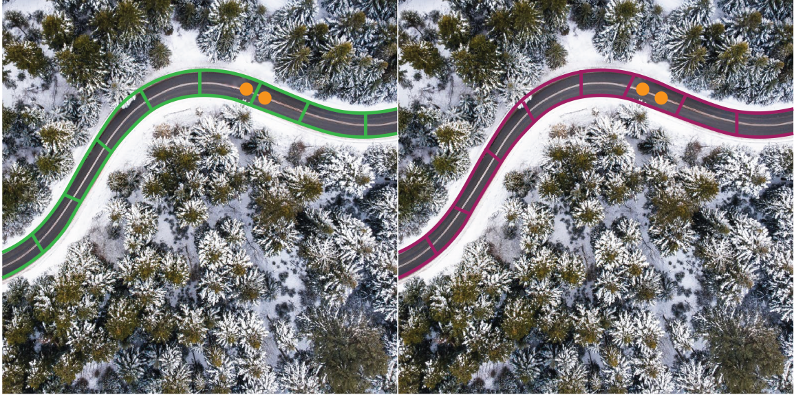
Figure 1-2: Two different, but equally valid ways to fit primitives to a winding road. Notice that while the two orange dots belong to different primitives on the green fitting, they belong to the same primitive on the purple fitting.
