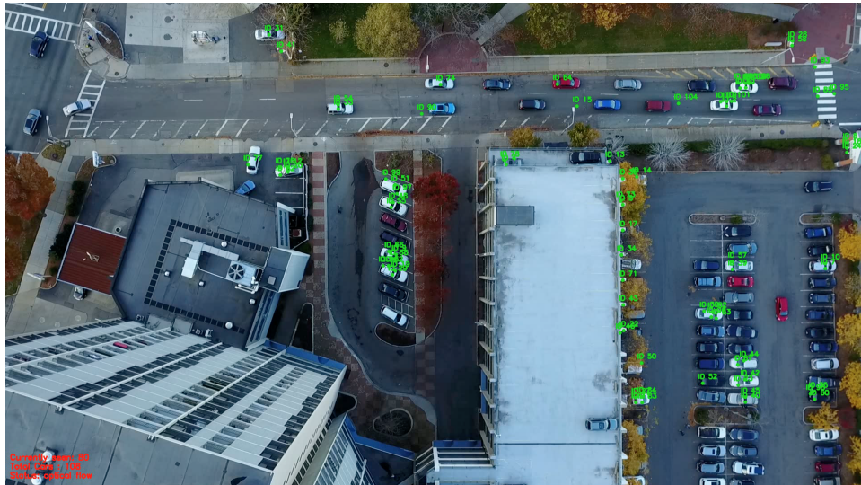
Figure A-1: Feature detection using sparse optical flow.
