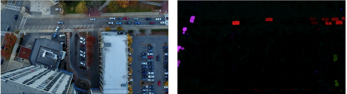
Figure B-2: RGB representation of flow vector field generated by Gunnar-Farneback method.
