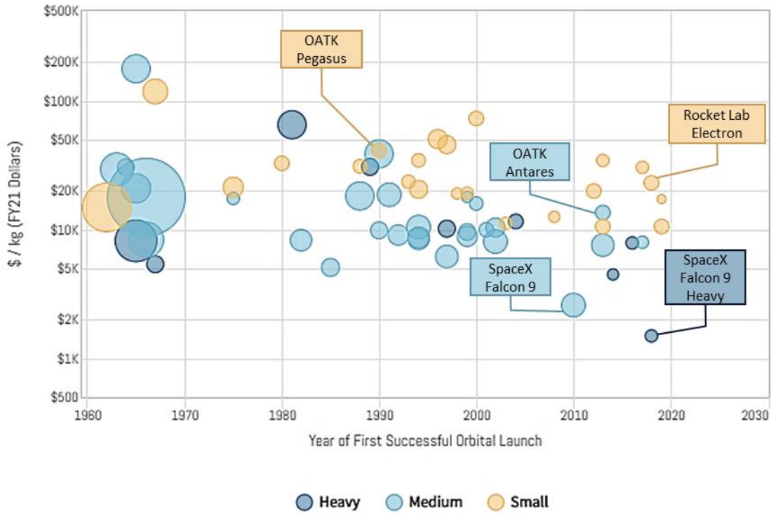
Figure 1-5 Cost of various launch vehicles per kg based on year of launch [11]
