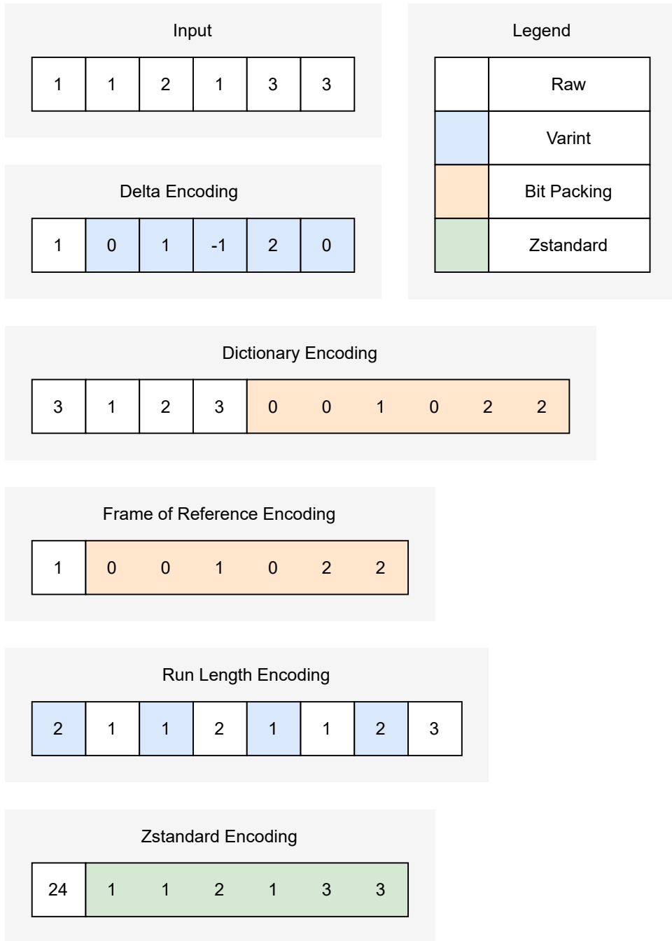
Figure 3-2: Layout of all encodings on a example input consisting of six uint32_t values. Note that the number of bytes occupied by each encoding is not represented by the size of the squares.
