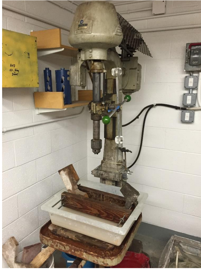
Figure 5.5 Picture of the coring machine.
