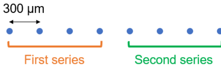
Figure 6.23 Schematic of the 6-hr micro-indentation test array. The eight indents form an array. Each blue circle corresponds to one indent.
