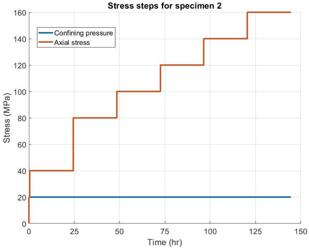
Figure 5.18 Stress steps for specimen 2.
