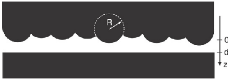
Figure 2.44 Schematic of Greenwood and Williamson's assumption for surface geometry (1966).
