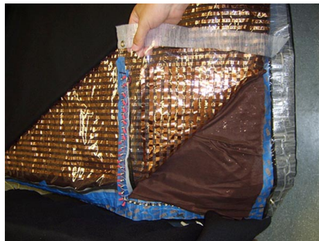
Figure 5-2: Pressure sensitive bedsheet from [83].
