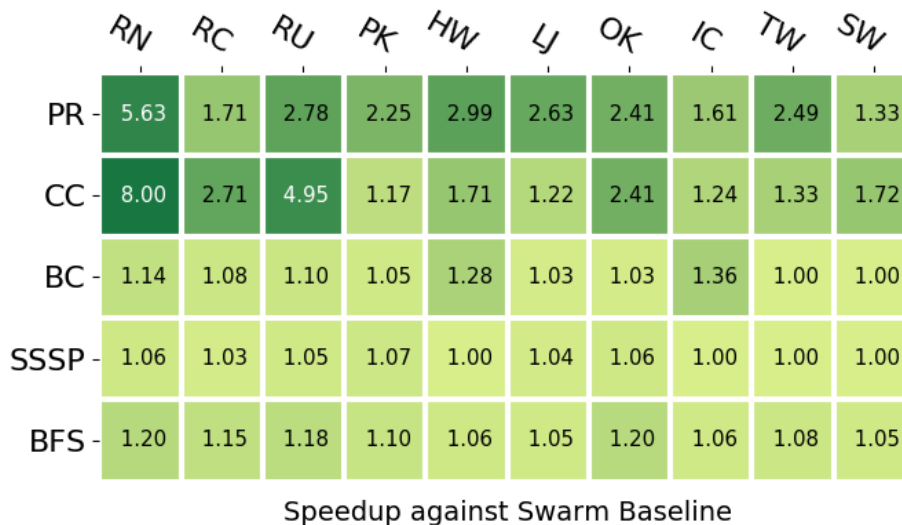
Figure 6-1: Heatmap of speedups of generated code from the Swarm GraphVM. Each cell reports the speedup of the optimized code over the Swarm baseline unoptimized version, with larger speedups in darker green. Columns correspond to graph inputs, and rows correspond to algorithms.
