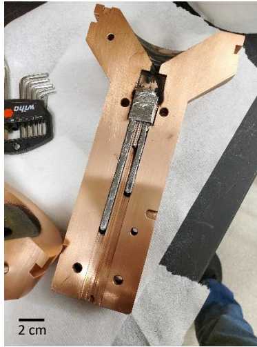
Figure 2.2: Alloy in water-cooled Cu mold after suction casting.
