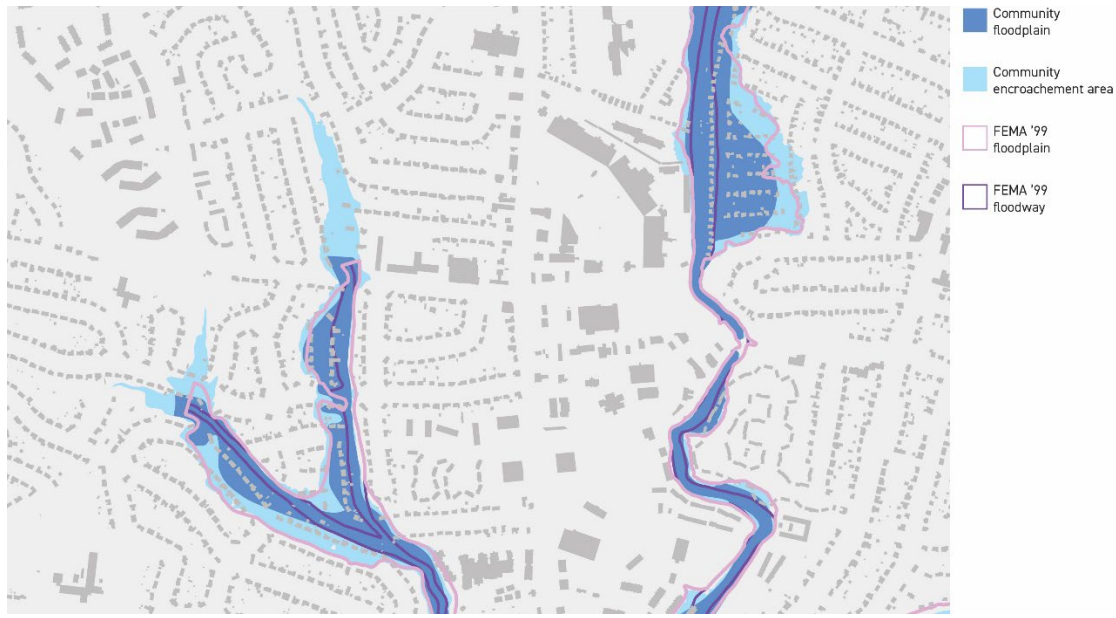
Figure 5: Spatial comparison of FEMA Maps in 1999 (Scanlon, 2020) and Community Map floodplains (Mecklenburg County GIS, 2019a-b)
