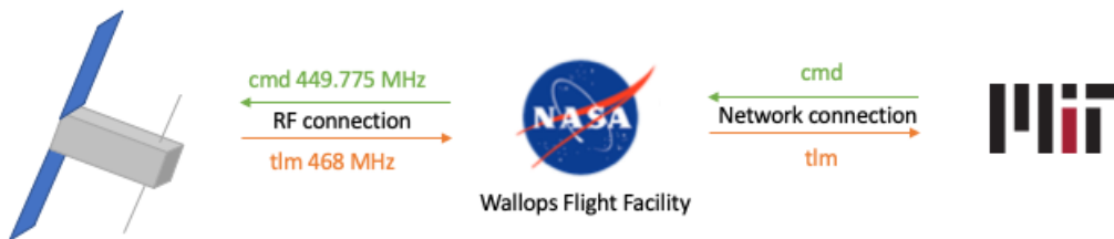
Figure 2-2: Diagram of the connection to and from the DeMi satellite via the Cadet radio. The NASA Wallops Flight Facility has a ground station antenna that is configured to interface with DeMi’s Cadet radio and route the telemetry and commands between the DeMi satellite and the MIT ground station.
