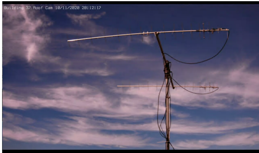
Figure 2-3: Image of the MIT ground station antenna on the roof of building 37. The MIT ground station uses a Lithium radio to communicate with the DeMi satellite with an uplink frequency of 449.775 MHz and a downlink frequency of 401 MHz.
