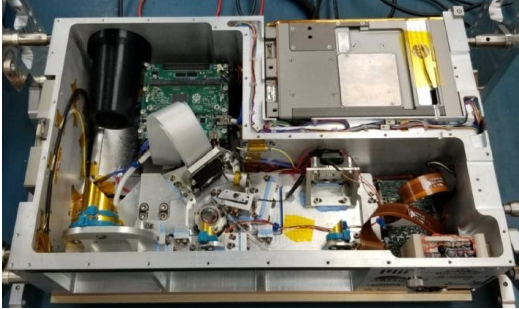
Figure 1-2: Image of the fully integrated spacecraft. The bus is the main box that houses all of the components and the bus electronics are in the top right corner, taking up about 1.5U of the spacecraft. The payload is housed in the remaining L-shaped volume. The spacecraft baffle, in black, is mounted to the top left of the internal volume. Next to the baffle is the payload electronics stack in green. The electronics stack includes the two Raspberry Pi compute modules and the DM driver boards. The payload optical bench is mounted in the lower part of the bus volume and the two camera boards are mounted to the right of the payload optical bench. This image is taken from [18].
