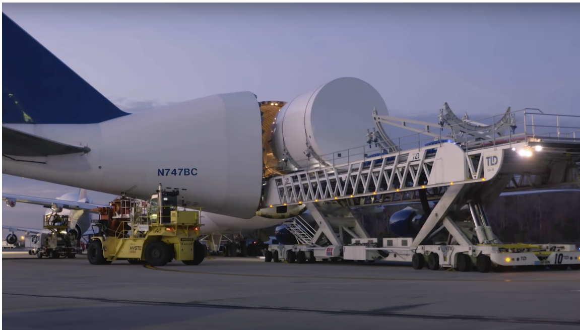
Figure 1-4: Cargo Loader docked on the open Swing Tail to load sub-assemblies
