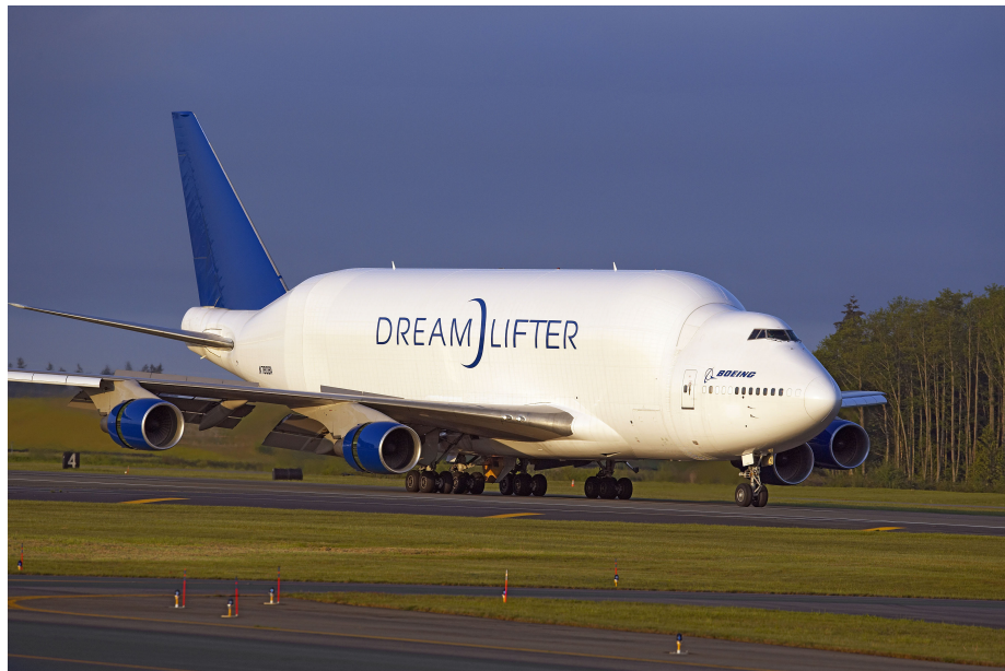
Figure 1-3: The bulging fuselage is a unique design feature of the Dreamlifters. Source: Boeing Media
