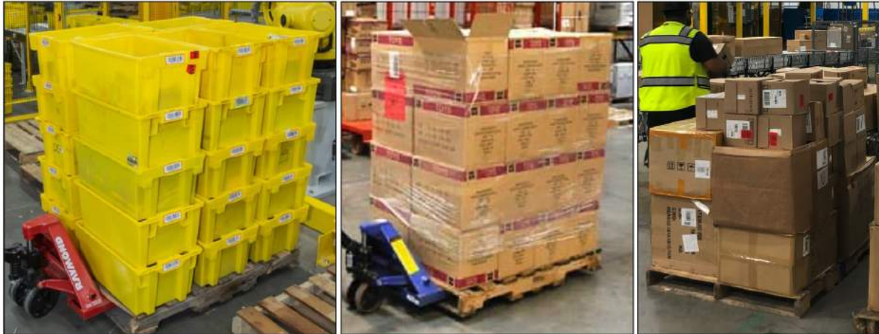
Figure 2-3: Left: A pallet of totes. Center: Single-SKU pallet. Right: Mixed-case pallet.
