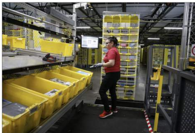
Figure 2-19: Amazon associate stowing inventory. The associate removes an item from one of the totes, scans the item, places it into an available cell in the inventory pod, and scans the cell location to record it virtually.
