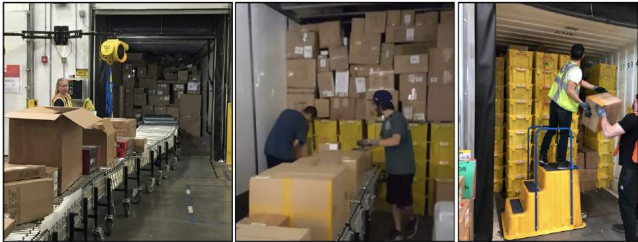
Figure 2-17: Various processes for unloading floor loaded trailers. Left: Unloading a section of cases using a powered flexible conveyor. Center: Unloading a hybrid floor load wall with both cases and totes. Right: Using a ladder to safely remove unstable containers that may have shifted during transit.
