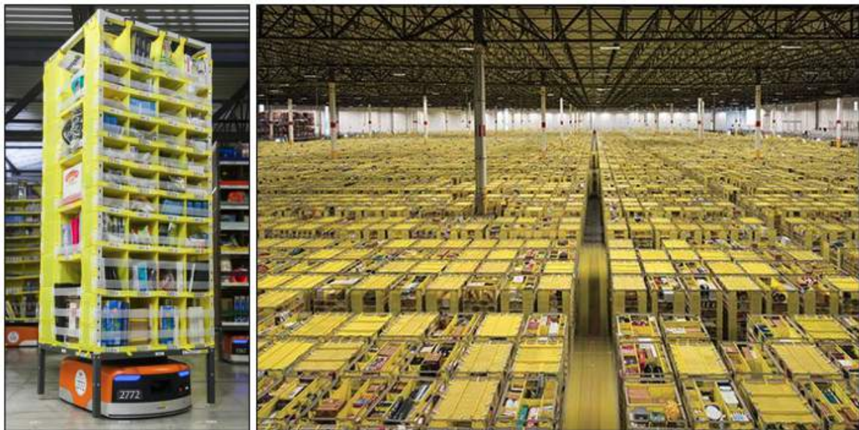
Figure 2-9: Amazon robotics inventory floor (right), where robotic drive units (left) transport densely-packed inventory pods to stow and pick stations located along floor edges. Photo credit: The New York Times.
