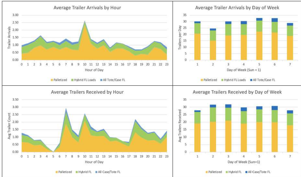
Figure 2-13: Average number of trailers arriving and received by a representative ARS FC, shown by hour and day of the week, and categorized by trailer load type. Top row shows distribution of arrivals (when trailers arrive at FC). Bottom row shows trailers received (when trailers are processed at a dock door).
