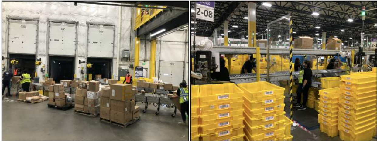
Figure 2-18: Left: Palletized cases are staged along the conveyor feeding the decant line as buffer material, to be injected when case flow from the trailer is disrupted. Right: Decant workers take cases from the middle (waist-height) accumulator line, remove items and place them into totes. Totes are dropped to the lower conveyor (ankle-height) for transport downstream. Empty corrugate is removed on the upper conveyor (overhead) to a compactor. Associates stand idle when there is an insufficient flow of work.
