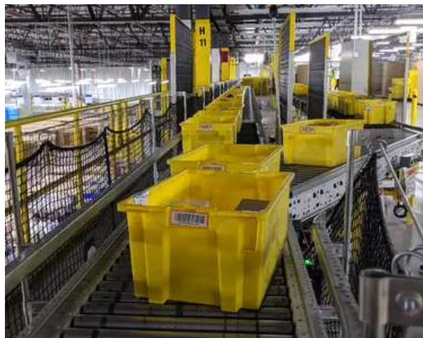
Figure 1-3: Amazon standard yellow totes, which can hold items up to 18" long, can be either nested or stacked, depending on orientation.
