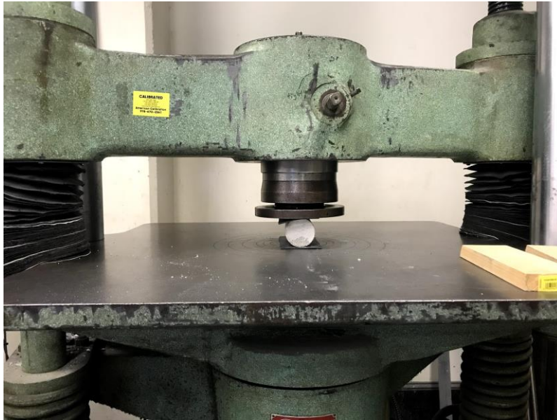
Figure A - 2: Actual splitting tensile test setup
