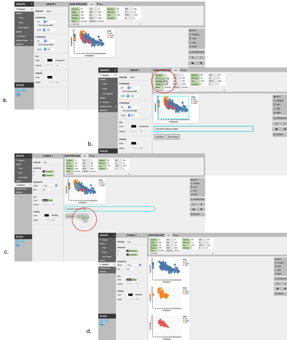
Figure 5-4: Process of applying a column facet to a group. Red circles added for clarity.
