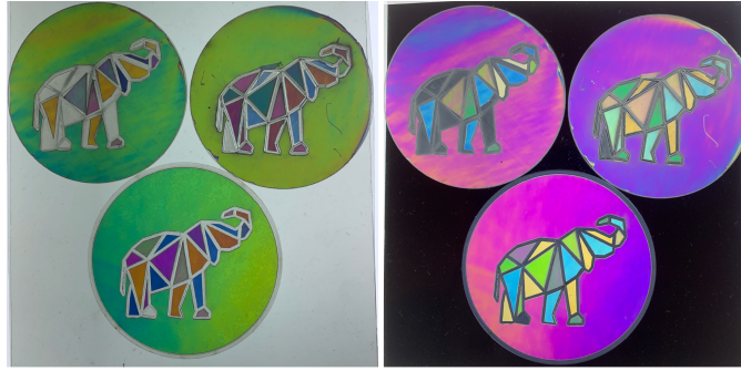
Figure 42: Comparison of the three methods between aligned and crossed polarizers. In the images going clockwise: group layering by color method, incremental layering without water method, and incremental layering with water method
