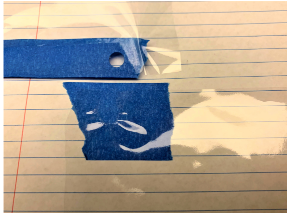
Figure 16: With the use of masking tape (top sheet), the resulting punched hole had clean edges and minimal surface texture irregularities. Without the masking tape (bottom sheet), the punched hole tore to the edge, which rendered it unusable, and had edge textural irregularities.
