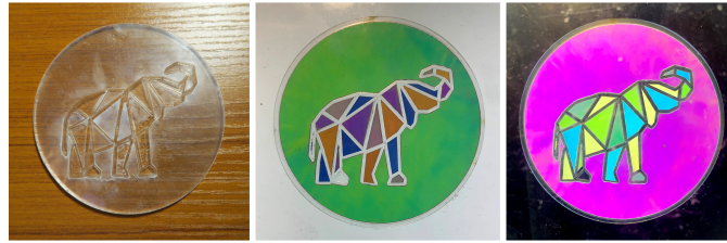
Figure 38: Fabrication results using the incremental layering method with water for the elephant image. In the colorless image, the white powdery dust was easily wiped off, and in the colored images, the shapes adhered well to the base board, had clear solid colors, and had minimal surface texture irregularities.
