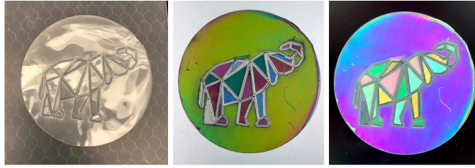
Figure 36: Fabrication result using the incremental layering without water method. From left to right: the colorless mosaic, mosaic between aligned polarizers, and the mosaic between crossed polarizers.
