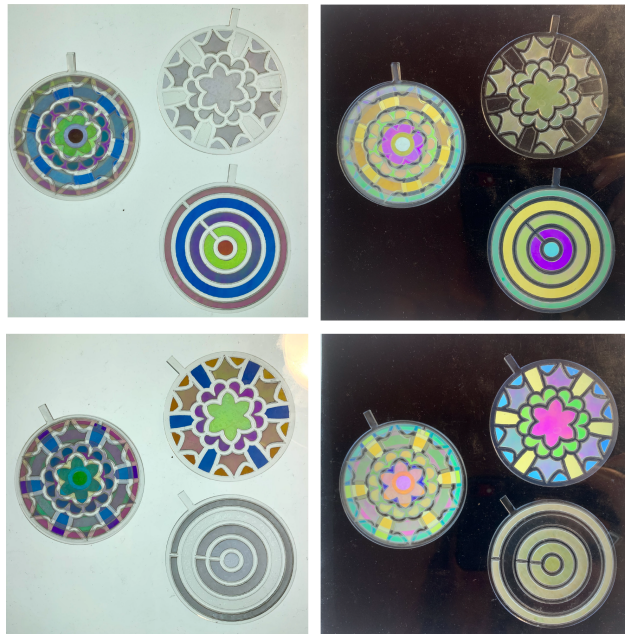
Figure 51: Demonstration of image visibility configurations. Top row: ring design is visible and the kaleidoscope pattern is not. Bottom row: kaleidoscope pattern is visible and the ring design is not. Left column: aligned polarizers. Right column: crossed polarizers.
