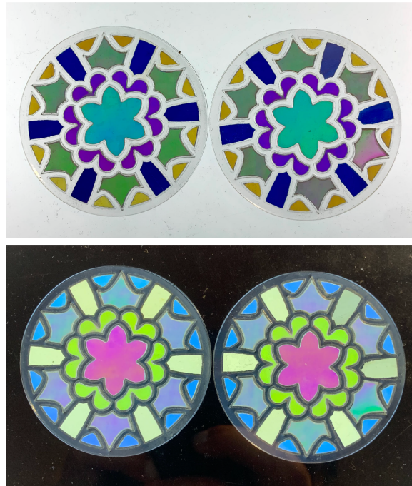
Figure 55: Individual lens mosaics without the third polarizer. Top: aligned polarizers. Bottom: crossed polarizers.
