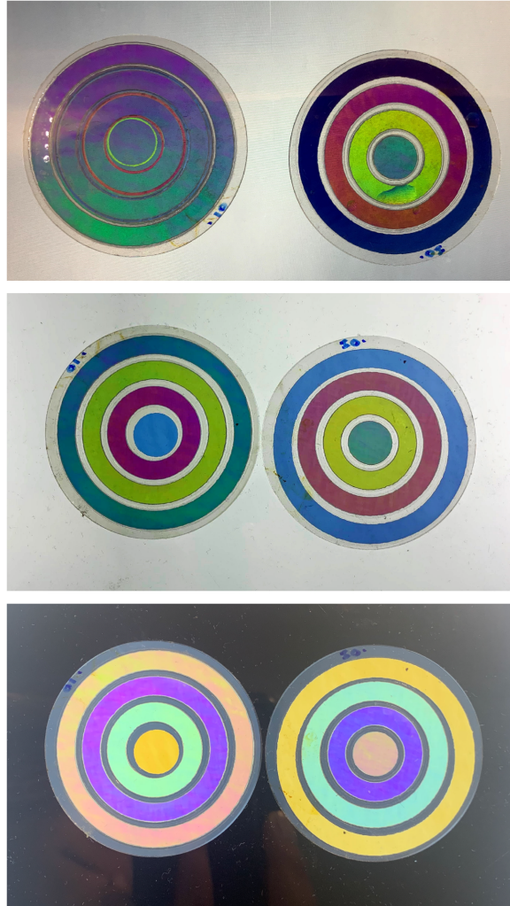
Figure 31: As shown in the top image, the design in which the color layers were ordered from inside to outside shapes required post processing to achieve the desired colors. The design in which surrounding (outside) shapes were cut before enclosed (inside) shapes, the desired colors were achieved without any post processing. The middle and bottom images show the designs with aligned and crossed polarizers, respectively.
