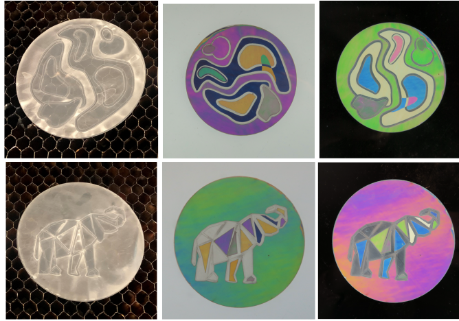
Figure 35: Fabrication result using the group layering by color method. From left to right, the columns exhibit the colorless mosaics, colored mosaics under aligned polarizers, and complementary colored mosaics under crossed polarizers.
