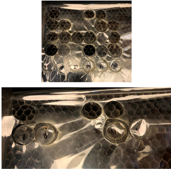
Figure 26: Cut results for lower power test settings at various speeds with a 1/16" wood top layer. Low power high speed settings did not cut through the cellophane on the first pass, and low power low speed settings caused edge melting and discoloration.
