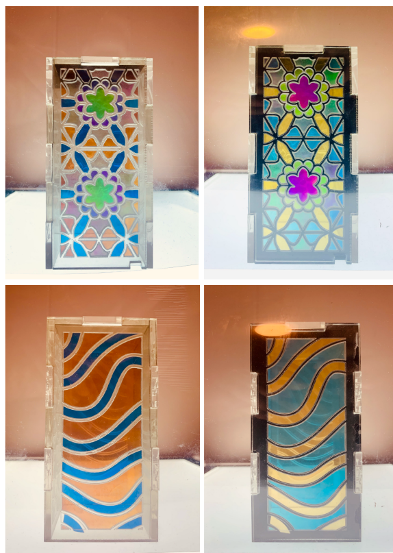
Figure 45: Color pattern of lantern walls with one outside polarizer. The left column shows the results of an aligned polarizer outside the lantern, and the right column shows the results of a crossed polarizer.
