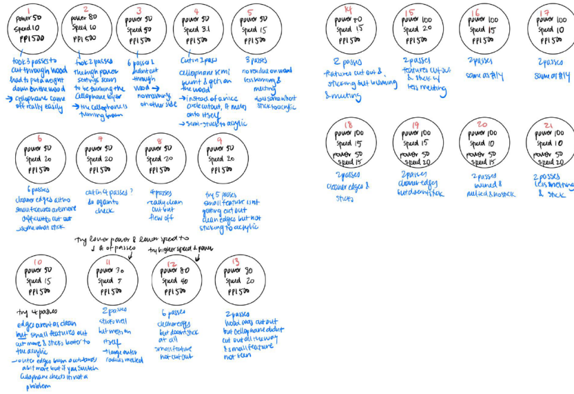
Figure 20: Test settings and observations with a 1/8" wood top layer.
