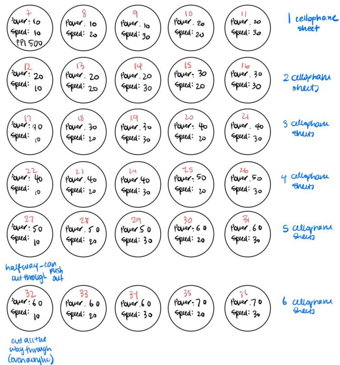
Figure 28: Water spray test settings and observations for a variety of cellophane layers to find the optimal power and speed settings
