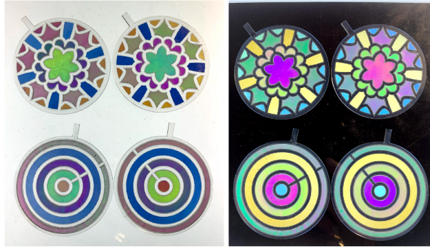
Figure 50: Individual lens mosaics for both designs. Left: aligned polarizers. Right: crossed polarizers.
