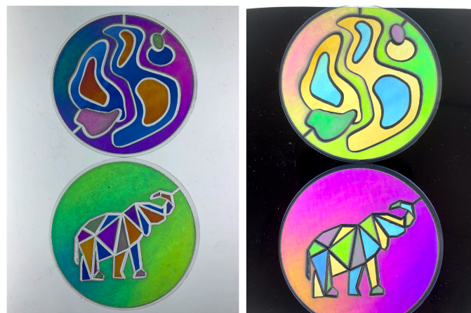
Figure 41: Fabrication results using the incremental layering method with water and slits in shapes enclosing other shapes.
