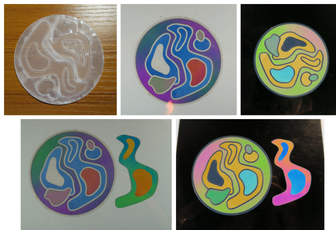
Figure 39: Since the outer shape was cut after the inside shapes, post processing was required. The missing gap of material exists because the shape was accidentally removed during fabrication.
