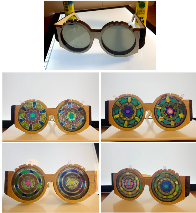
Figure 52: Sunglasses result with two morphing images. Top image: no mosaic lens. Top row: ring design is visible and the kaleidoscope pattern is not. Bottom row: kaleidoscope pattern is visible and the ring design is not. Left column: aligned polarizers. Right column: crossed polarizers.
