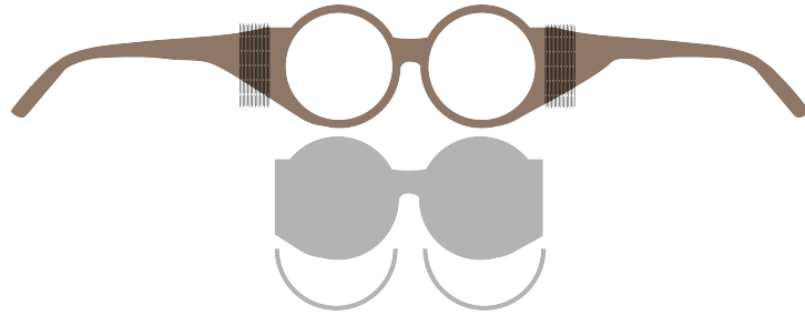
Figure 54: Wood frame design for the sunglasses with a third polarizer. The brown represents 1/8" wood, and gray represents 1/16" acrylic.
