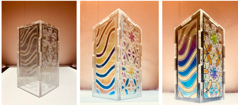
Figure 46: Lantern with no outside polarizer, aligned polarizer, and crossed polarizer.
