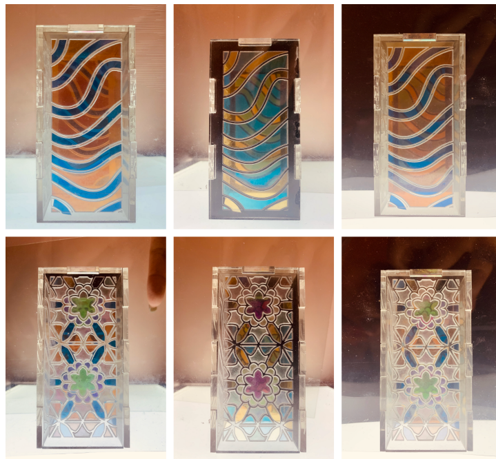
Figure 47: Different wall color configurations made with two outside polarizers. From left to right: aligned outside polarizers that are both aligned with the inner polarizer, aligned outside polarizers that are both crossed with the inner polarizer, and crossed outside polarizers.
