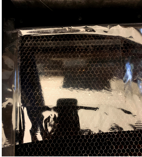
Figure 17: Air gaps in the cellophane at the top and left border of the cutting table. Since the cellophane sheet does not lie flat at the edges of the cutting table, those areas should be avoided to minimize surface irregularities and maximize cellophane adhesion to the acrylic base board.
