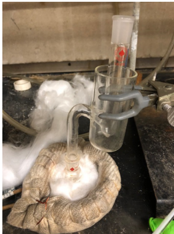
Figure 3.5: (Left) Schematic representation of water distillation apparatus. (Right) Picture of water distillation apparatus.
