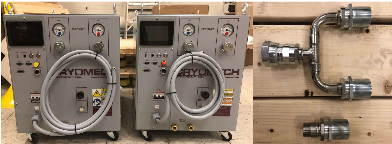
Figure 5.7: Helium compressors (left) and Aeroquip adapters (right) for helium recirculation system.
