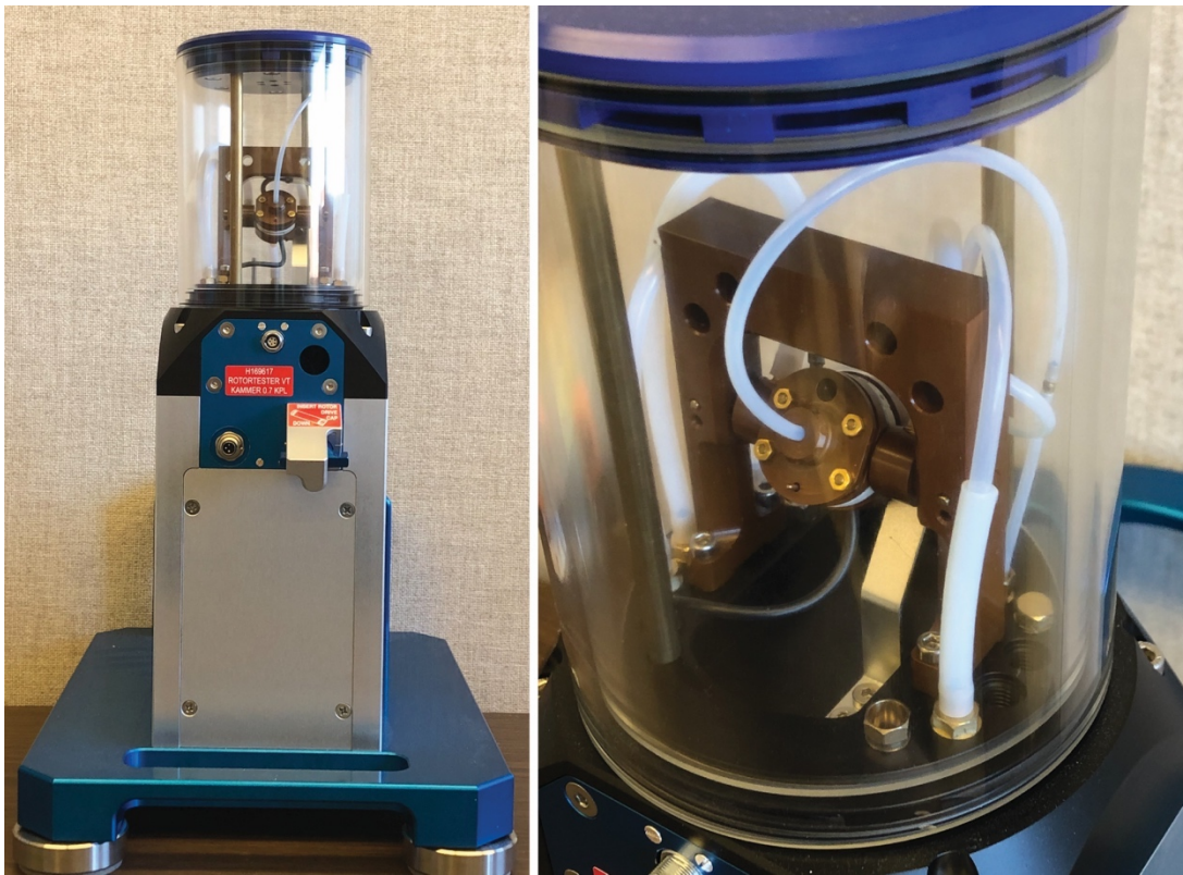
Figure 6.13: Bruker test stand equipped with 0.7 mm stator. The test stand can be used for destructive testing of diamond rotors.
