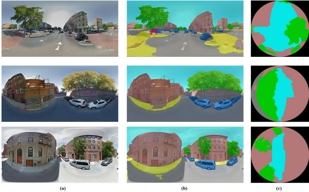
Figure 2. The segmentation of street-level images using a deep learning algorithm, demonstrating (a) the raw Google Street View panoramas, (b) the blend of the segmentation results on Google Street View panoramas, and (c) the segmented hemispherical images.
