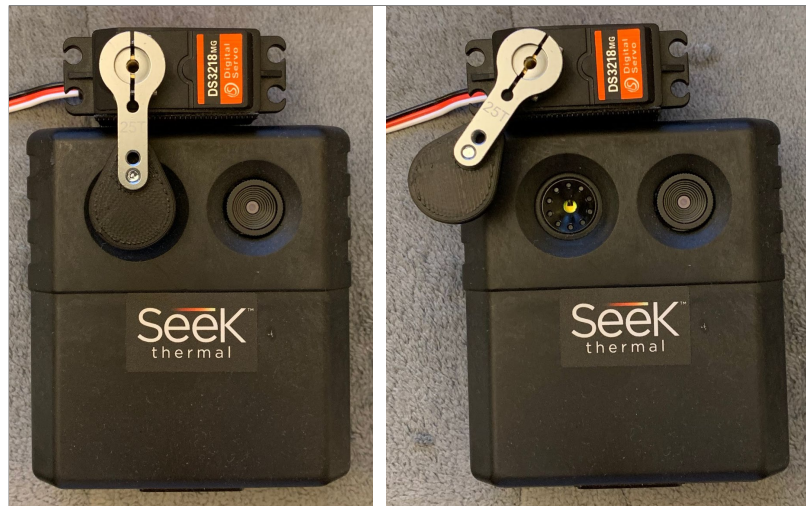
Figure 2-7: Seek Scan shutter mechanism.
