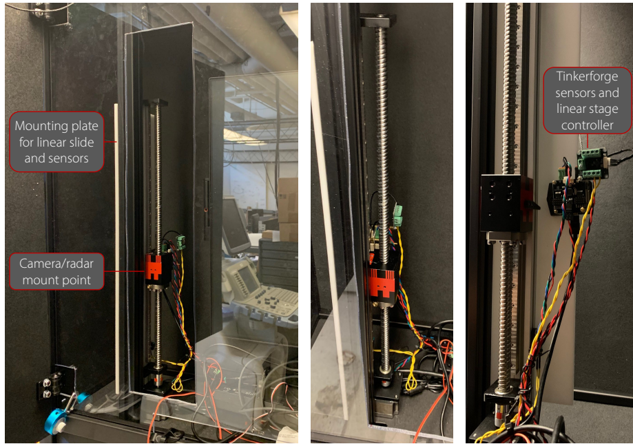
Figure 2-11: Sensor and linear stage controller layout on mounting plate.
