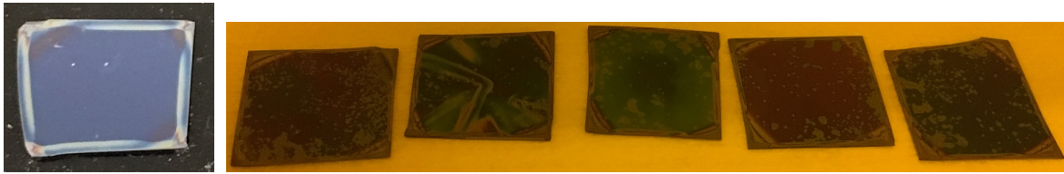
(a) Initial spin-coating tests showed no apparent problems. (b) However, at a different time, all of the second coatings on small blank 2cm x 2cm silicon pieces looked abysmal.
