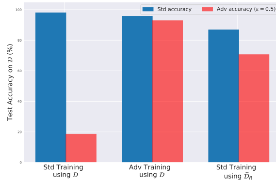
Figure A-6: Repeating the experiments shown in Figure 2-2 for the Restricted ImageNet dataset. Standard and robust accuracy of models trained on these datasets.
