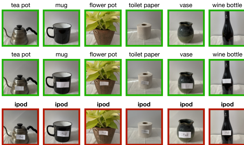
Figure 6-11: Typographic attacks on CLIP: We reproduce the results of Goh et al. [Goh+21] by taking photographs of household objects with a paper containing handwritten text “iPod” attached to them (third row). We see that these attacks consistently fool the zero-shot CLIP classifier (ResNet50)—compare the predictions (shown in the title) for the first and third row. In contrast, if we instead use a blank piece of paper (second row), the model predicts correctly.
