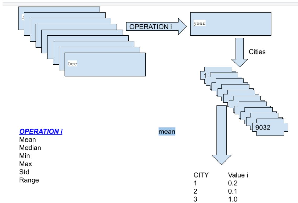
Figure 3-3: Example of Satellite image data processing . To top left, different rasters for different months are aggregated into a single raster for each year aggregated with either mean, median, max, min, std values of the months for each point on raster. Then year raster is clipped into 9000+ different city rasters which are then further processed to give one or more values for each city
