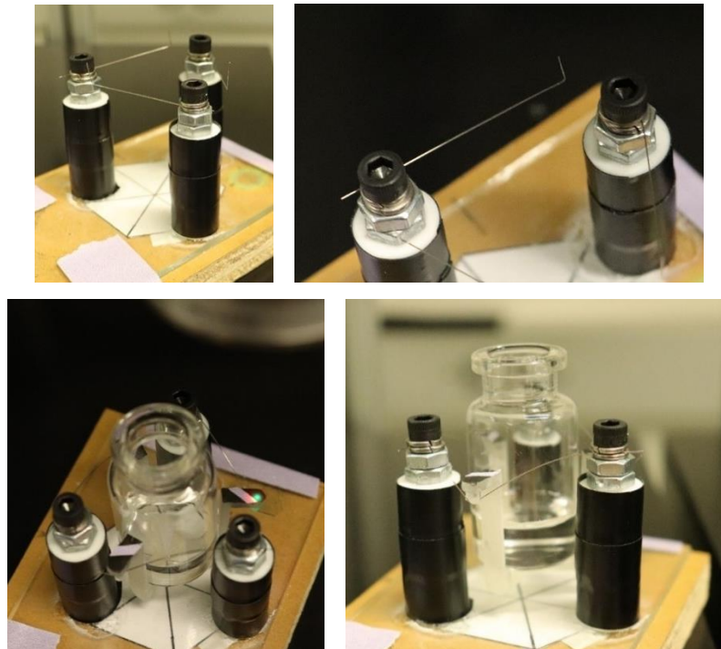
Figure 15: Straight Spring with High Mounting and Right-Angle Hard Stops Experimental Setup.
