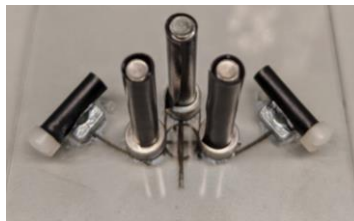
Figure 18: Wire Bending Template.
