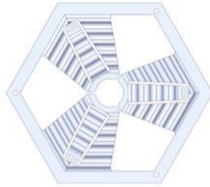
Figure 38: The Final Prototype 3D Printed Diaphragm Design.
