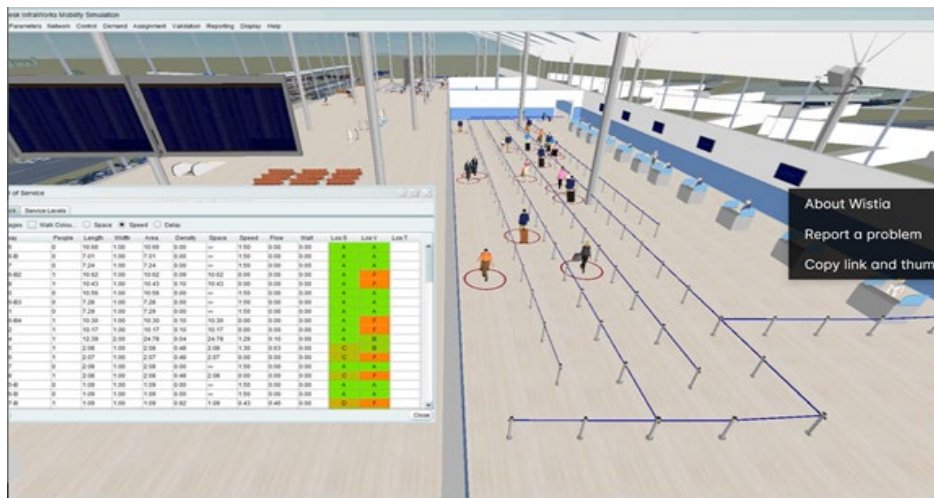
Fig. 2.9. From: https://www.autodesk.com/campaigns/aec-return-to-workplace# , revised July 2021. The picture shows the ABM implementation of the Autodesk software company in the Revit BIM application. The image shows their simulation of social distancing in the workplace, called “Return to the Workplace,” launched in 2021.
