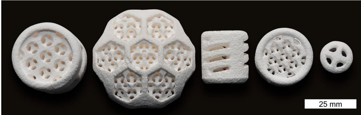
Figure 1.3: Sample geometries of parts fabricated using binder jet additive manufacturing and aluminum oxide powder for use in catalysis (image from Johnson Matthey [15]).
