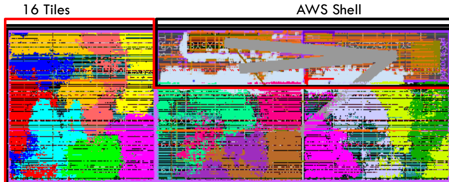
Figure 3-9: FPGA layout of the 16-tile Chronos sssp accelerator. Each Chronos tile is shown in a different color.
