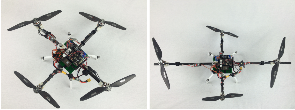
Figure 3-8: Optimizing a quadcopter with flight time metric and geometry constraints. Left: a standard quadcopter. Right: optimized rectangular quadcopter.
