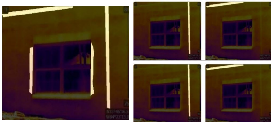
Figure 4-25: Left, Input segmented anomaly, right, output categorized anomalies after using the BFS algorithm.
