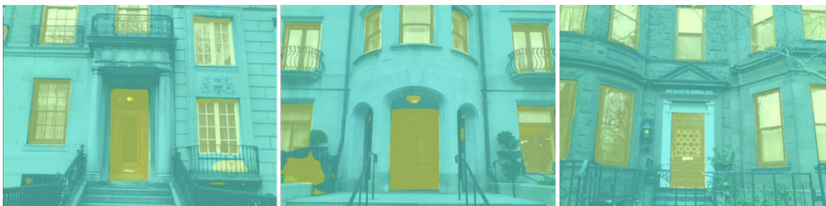
Figure 4-23: Results from the PSPNET algorithm with segmented façade elements (walls, windows).
