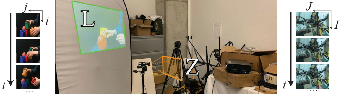
Figure 4-2: Scene geometry adopted in computational mirrors [3]. The observed scene can be written as a product of the hidden scene and the light transport. Figure courtesy of [3].
