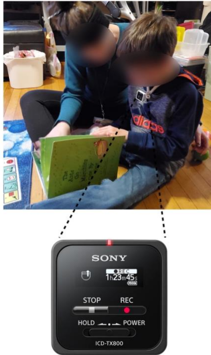
Figure 17: Data was collected using a small audio recorder (Sony IDC-TX800) that could be attached magnetically to participants' clothing. The recorder was easy to use during day-to-day activities, like reading.
