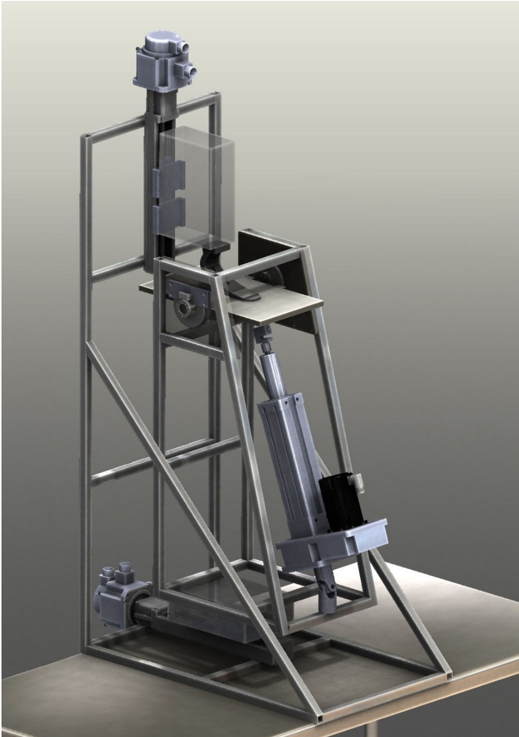
Figure 4-1: A rendered CAD image of the PFTD and prosthetic foot.
