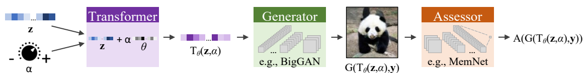
Figure 3-1: Schematic of the model. The model learns how to transform a z vector such that when fed to a Generator, the resulting image’s property of interest changes. The transformation is achieved by the Transformer , who moves the z vector along a learned direction, \theta , in the Generator’s latent space. An Assessor module (e.g., MemNet) predicts the property of interest (e.g., memorability). Finally, \alpha acts as a knob to set the desired degree of change in the Assessor value (e.g., MemNet score), telling the Transformer how far to move along \theta .
