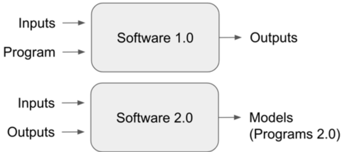
Figure 1-1: Comparing the I/O structure of software 1.0 vs software 2.0. In software 1.0, programmers provide inputs and the explicit instructions to be performed on those inputs to produce outputs. In contrast, software 2.0 consumes examples of inputs and outputs and must produce models that have learned the rules of the desired program.
