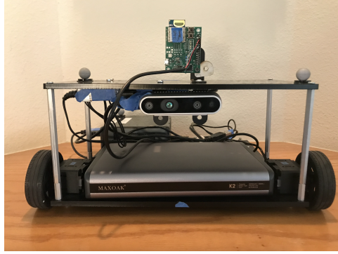
(a) Tag antenna aligned with the front of the robot to collect the front-facing antenna data set.
