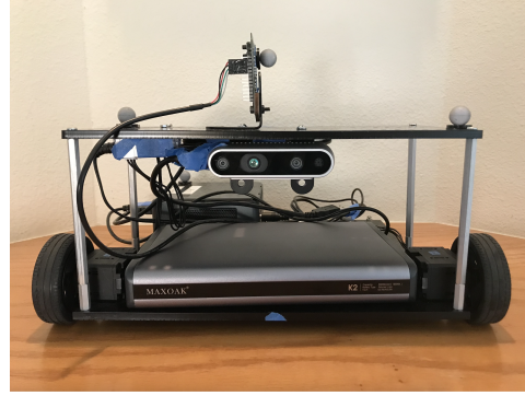
(b) Tag antenna 90 degrees offset from the front of the robot to collect the right-facing antenna data set. (Antenna is facing to the left in the photo.)
