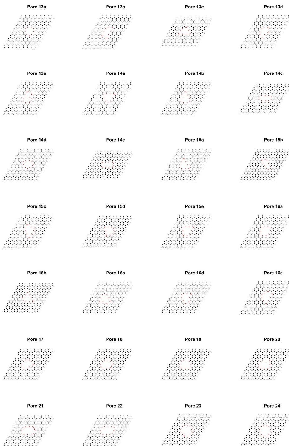
Figure 2-19. Atomic Structures of the hydrogen-terminated pores investigated. The pore size ranges from 13 to 24. Black dots represent carbon atoms, and red dots represent hydrogen atoms.
