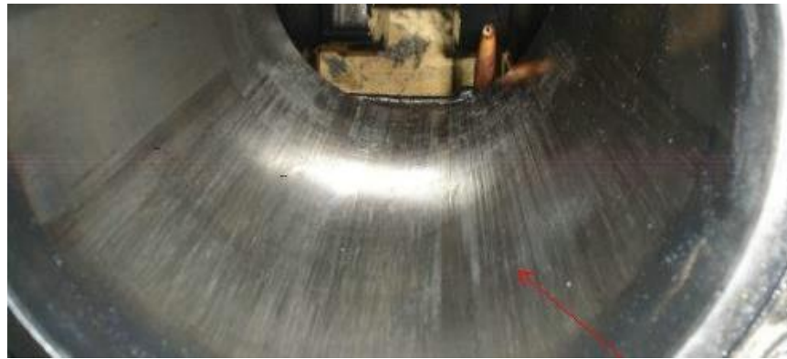
Figure 1.5. a cylinder liner with tribological failure
