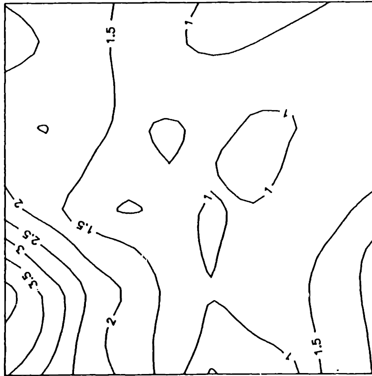
Figure 7.42: Shear Strain Distribution for Test DSC32 at \sigma'_{vc}=0.878 ksc.
