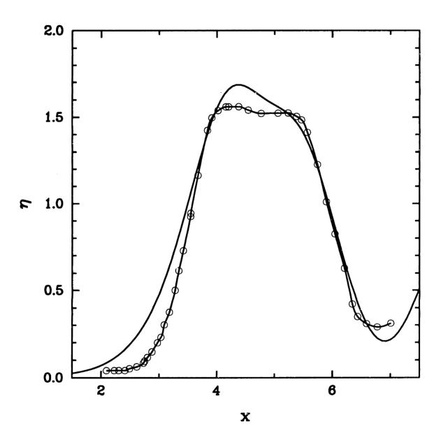
FIGURE 2.4 Profiles of leading waves (along the centerline) of undular bores; comparison of theory with experiments of Sandover & Taylor (1962); ——: theory,— $\ominus$ —: experiment. (a)  $\theta = \frac{1}{4}\pi$ , T = 12.5; (b)  $\theta = \frac{1}{3}\pi$ , T = 9.5
