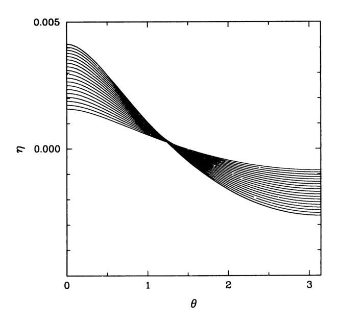
FIGURE 4.2 Intersections of the free-surface elevation of the computed nonlinear edge wave with planes of constant s. (a)  $H=0.1,\,\sigma=0.5,\,\epsilon=5.37\times 10^{-2};$  (b)  $H=0.1,\,\sigma=0.1,\,\epsilon=3.18\times 10^{-2};$
