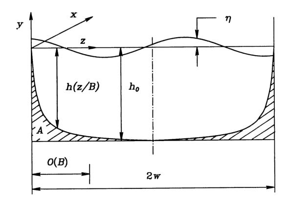
FIGURE 2.1 Channel cross-section.
