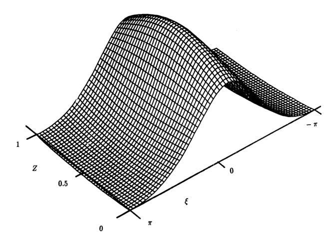
FIGURE 2.10 Wave of permanent form of period  $2\xi_0=2\pi$ , speed c=1.5, channel width 2W=1 and  $\mathcal{A}=-1$ .
