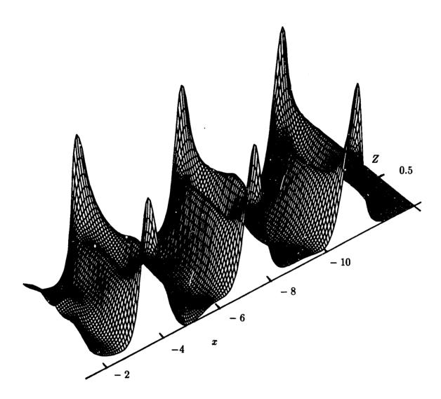
FIGURE 2.5 Upstream waves excited by transcritical forcing in channels with sloping sidewalls, at T=4 and  $p_0=10$ . (a)  $\mathcal{A}=0.5$ ,  $\lambda=-0.5$ , (b)  $\mathcal{A}=1$ ,  $\lambda=-1$ .
