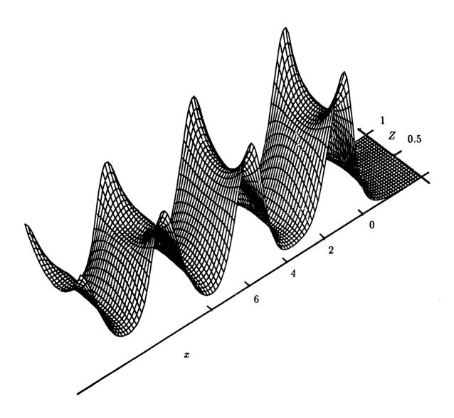
FIGURE 2.2 Computed free surface of the head of undular bores in channels with sloping sidewalls. (a)  $\theta = \frac{1}{4}\pi$ ,  $\eta_{\infty} = 1.08$ , T = 12.5; (b)  $\theta = \frac{1}{3}\pi$ ,  $\eta_{\infty} = 1.13$ , T = 9.5.
