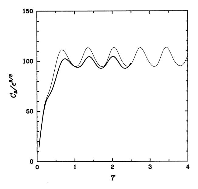
FIGURE 2.9 Variation of wave-resistance coefficient  $C_D$  with time T for  $p_0 = 10$ ;  $\dots : \mathcal{A} = 0; \dots : \mathcal{A} = -1 \ (\lambda = 1)$ .
