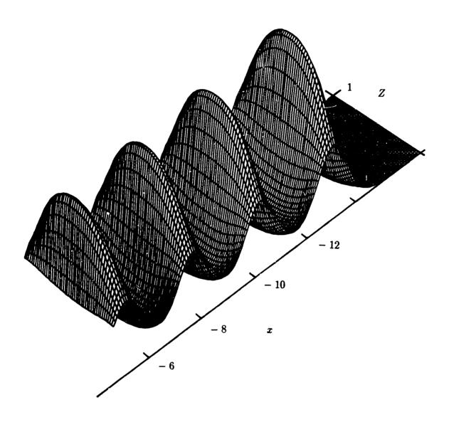
FIGURE 2.8 Upstream waves excited by transcritical forcing in channels with sloping sidewalls, at T=4 and  $p_0=10$ . (a)  $\mathcal{A}=-0.5$ ,  $\lambda=0.5$ , (b)  $\mathcal{A}=-1$ ,  $\lambda=1$ .
