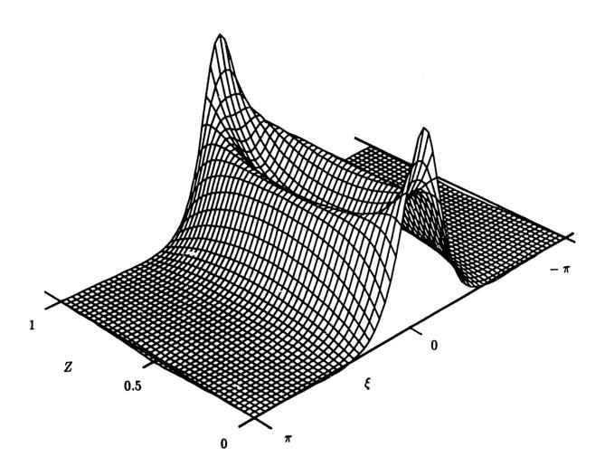
FIGURE 2.7 Periodic waves of permanent form of period  $2\xi_0=2\pi$ , speed c=2.5 and channel width 2W=1. (a)  $\mathcal{A}=0.5$ ; (b)  $\mathcal{A}=1.0$ .
