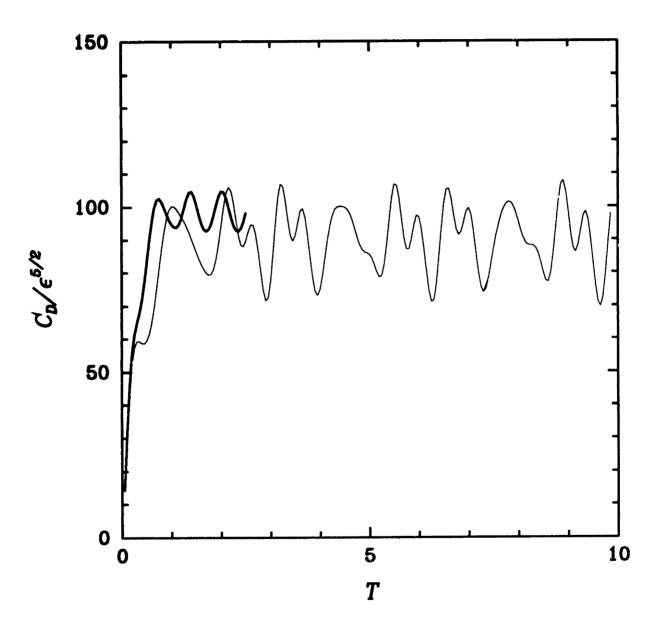
FIGURE 2.6 Variation of wave-resistance coefficient  $C_D$  with time T for  $p_0 = 10$ . (a)  $\longrightarrow$  : A = 0;  $\longrightarrow$  : A = 0.5 ( $\lambda = -0.5$ ). (b)  $\longrightarrow$  : A = 0;  $\longrightarrow$  : A = 1 ( $\lambda = -1$ ).
