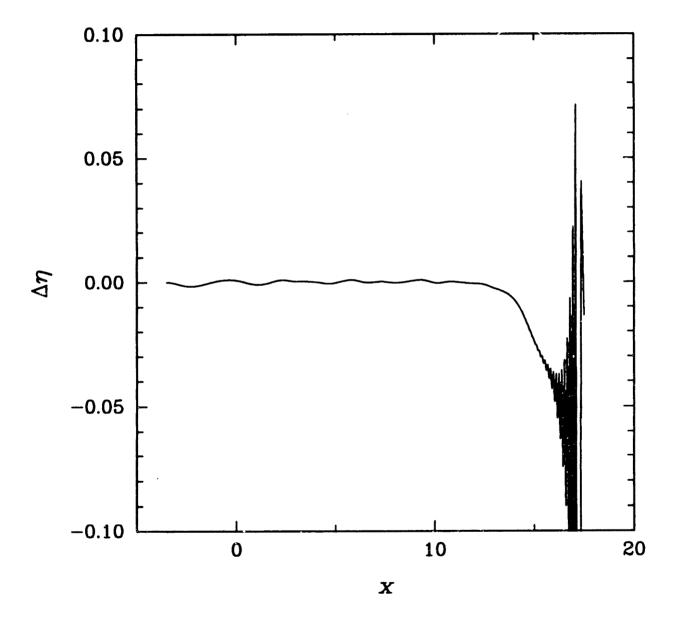
FIGURE A.1 Contamination at the downstream boundary at T=5 for  $\mathcal{A}=0.5$  and  $\eta_{\infty}=1$ .
