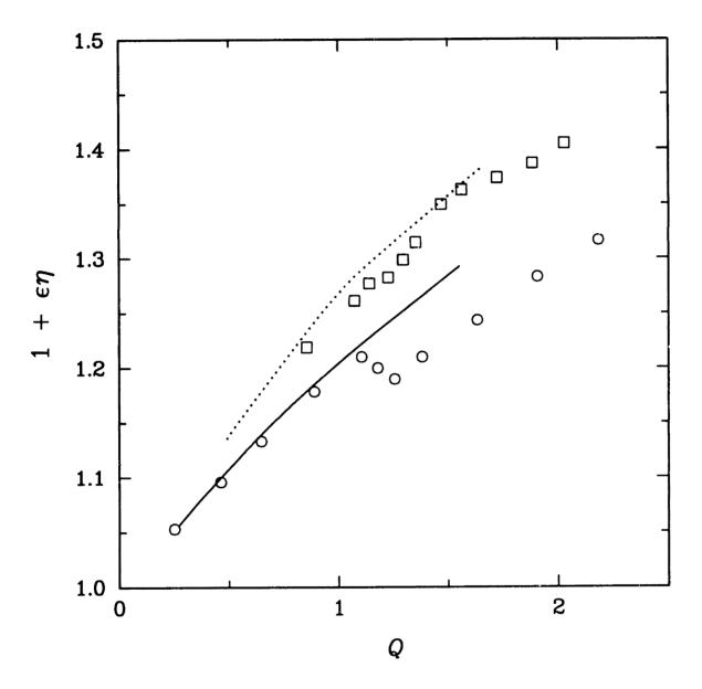
FIGURE 2.3 Variation of wave height of the leading crest (at the centerline) of undular bores with discharge; comparison of theory with experiments of Sandover & Taylor (1962), for two sidewall inclinations  $\theta$ ; ....: theory,  $\theta = \pi/4$ ;  $\square$ : experiment,  $\theta = \pi/4$ ; ...: theory,  $\theta = \pi/3$ ; o: experiment,  $\theta = \pi/3$ .
