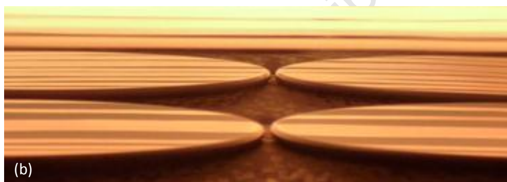
Figure 17. (a) Top view and (b) side view of silicon wafers being coated with a polycrystalline diamond film in a hot filament CVD reactor. Deposition areas as large as 400x1180 mm (0.5m 2 ) have been coated with this technology. Photo courtesy of Neocoat SA. [51] <qry> Author: did you ask for permission to use this images?<qry>
