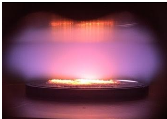
Figure 4. Diamond powder during H-termination in a hydrogen plasma at ~ 60 Torr of H 2 . The powder is initially heated by the plasma to ~1000°C for 10 min to degas the powder and then H terminated for 60 min at ~800°C. [12]
