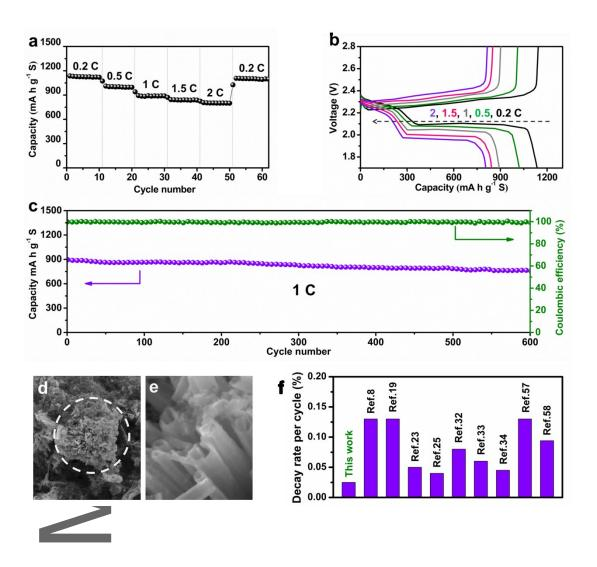
**Figure 5** Electrochemical performance of the  $S@Co_9S_8$  nanocomposite. a) Rate capabilities and b) discharge-charge curves at 0.2, 0.5, 1, 1.5 and 2 C. c) Cycling performance at 1 C over 600 cycles. d,e) FESEM images of the  $S@Co_9S_8$  composite after cycling. f) Comparison of the decay rate per cycle with other Li-S cathode materials reported in the literature.
