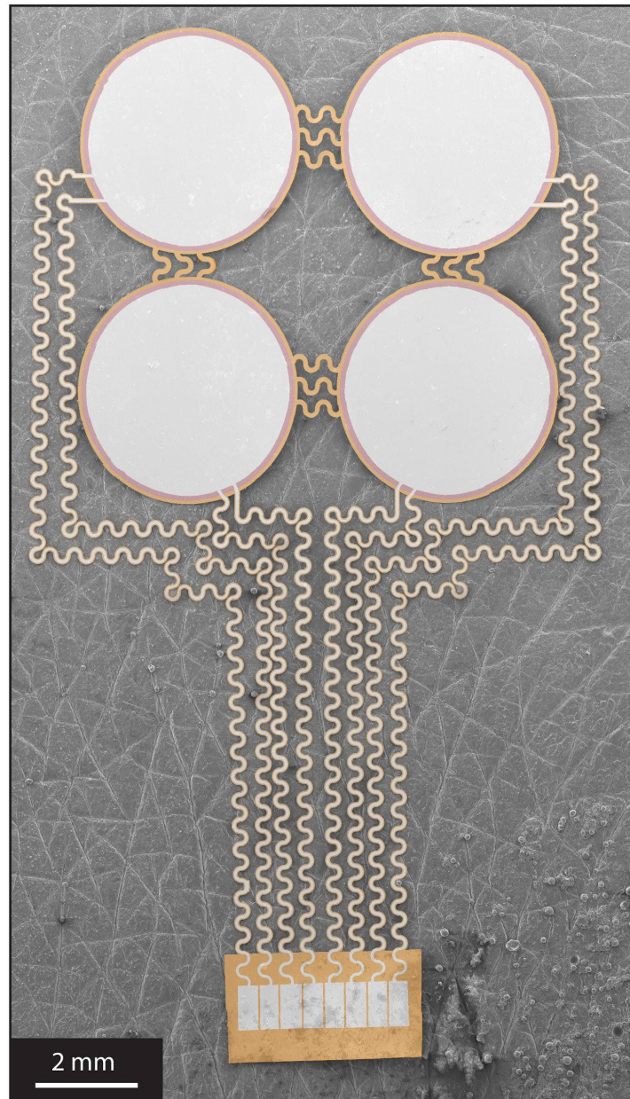
Fig. S4. Colorized SEM image of a cFaCES on a mock skin.
