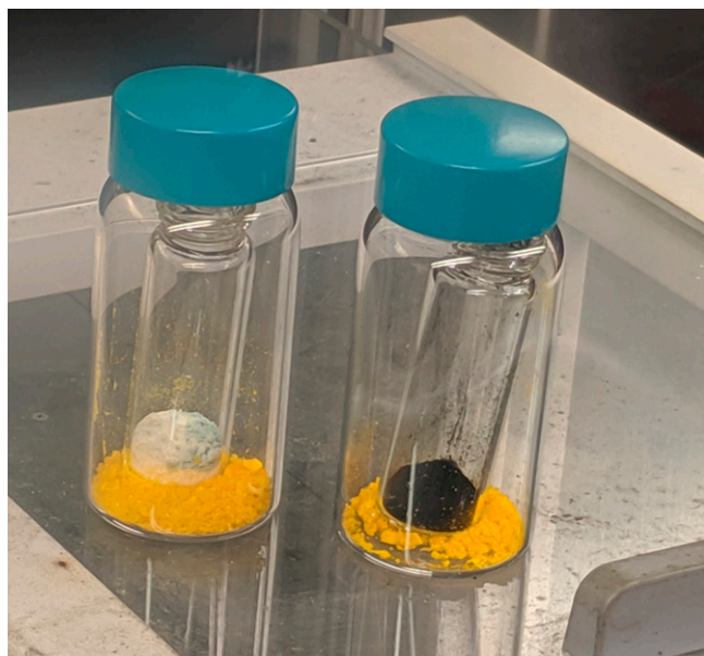
Fig. 1. The vapor-diffusion setup used to prepare [\text{Li}_2\text{O}_2]_{0.3} \cdot [\text{LiO}_2]_{0.7} \cdot \{\text{Li}[p\text{-C}_6\text{H}_4\text{O}_2]\}_{0.7} . The setup consists of a small vial that contains \text{Li}_2\text{O}_2 sealed within a larger vial containing p\text{-C}_6\text{H}_4\text{O}_2 . The vial on the left is a freshly prepared sample, while the vial on the right has been allowed to stand at room temperature for a month.
